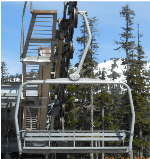
A1871 Quad Hanger Installed at Mt Baker Lift #8
