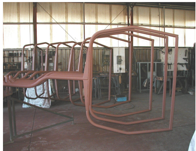
CH-43A Hangers on our Paint Carousel
